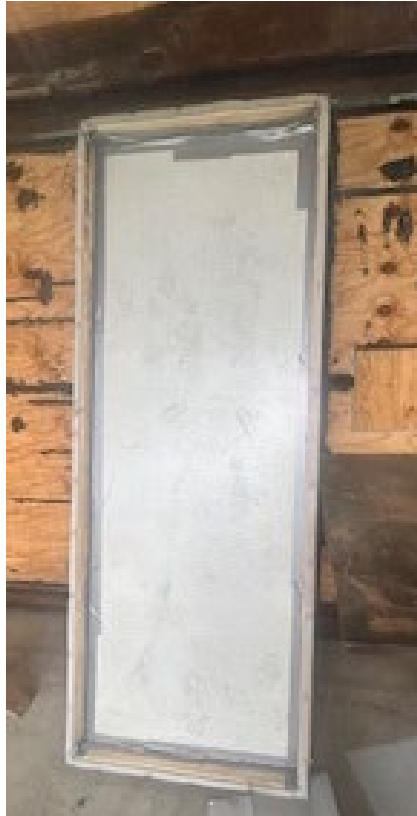
Photo No. 1 Armorcore UI 752 Level 1 Panel
