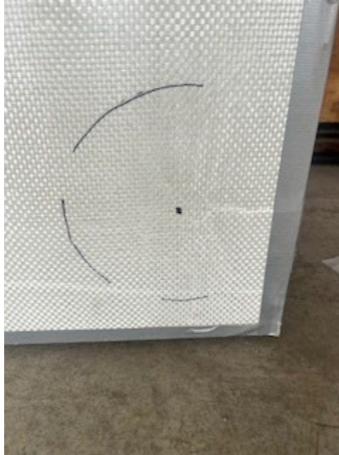
Photo No. 3 Armorcore UI 752 Level 1 Panel Impact 2
