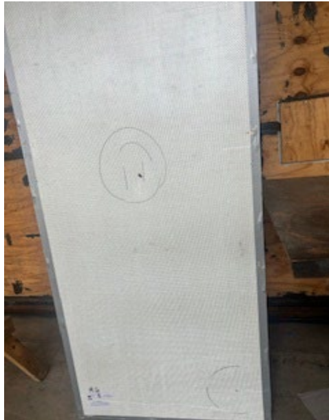
Photo No. 2 Armorcore UI 752 Level 1 Panel Post Impact
