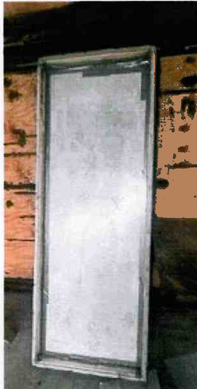
Photo No. 1 Armorcore UI 752 Level 1 Panel
