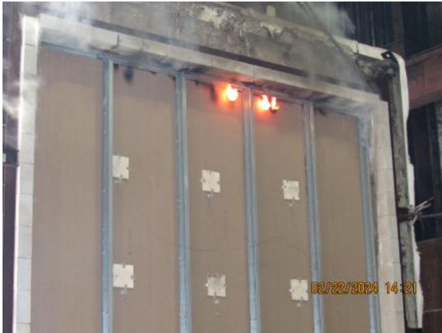
Photo No. 10 Flames on Top Perimeter
