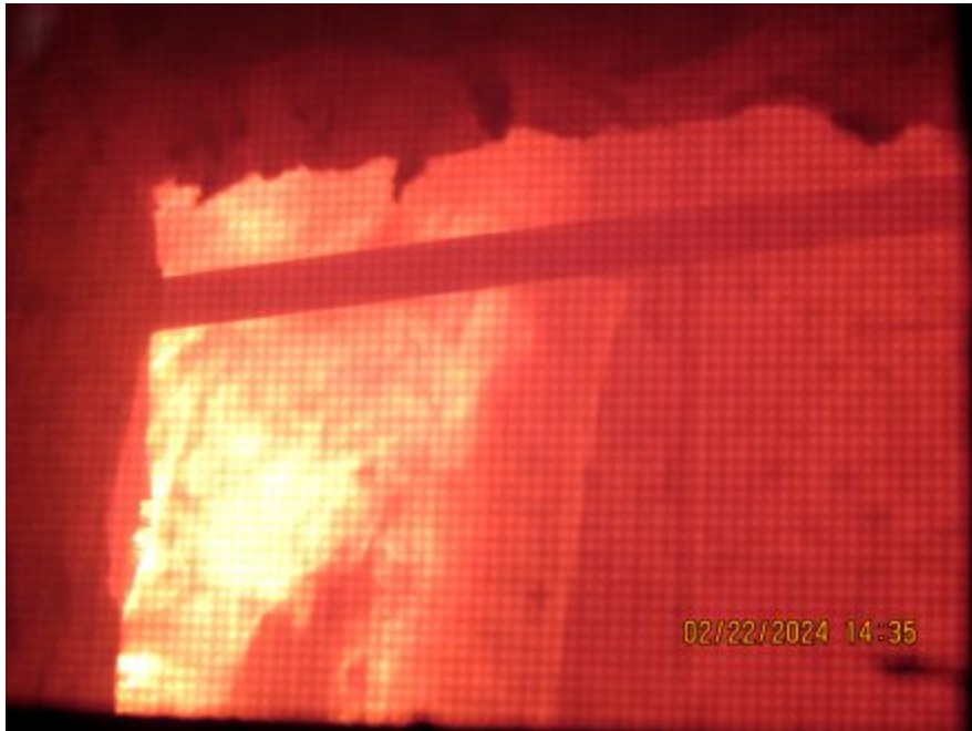
Photo No. 12 Increase of Flame in Exposed Side
