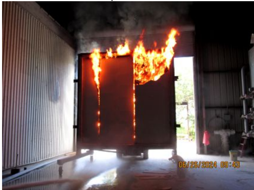
Photo No. 26 View of Exposed side Post-Test
