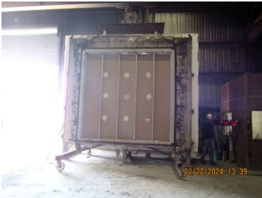
Photo No. 6 Unexposed side with TCs
