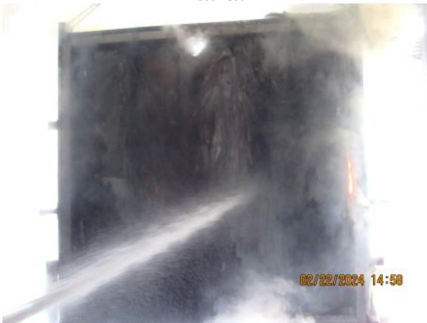
Photo No. 14 Sample During Hose Stream
