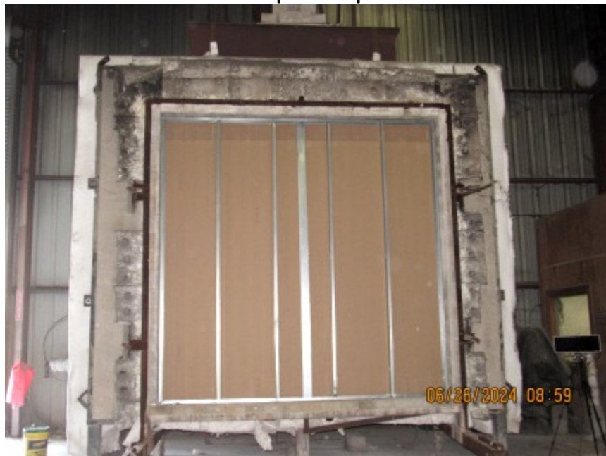
Photo No. 24 View of Hose Stream Re-Test Sample During Test
