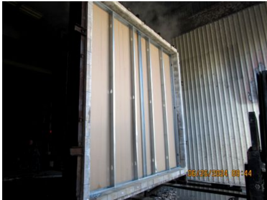
Photo No. 30 Post Hose Stream Re-Test
