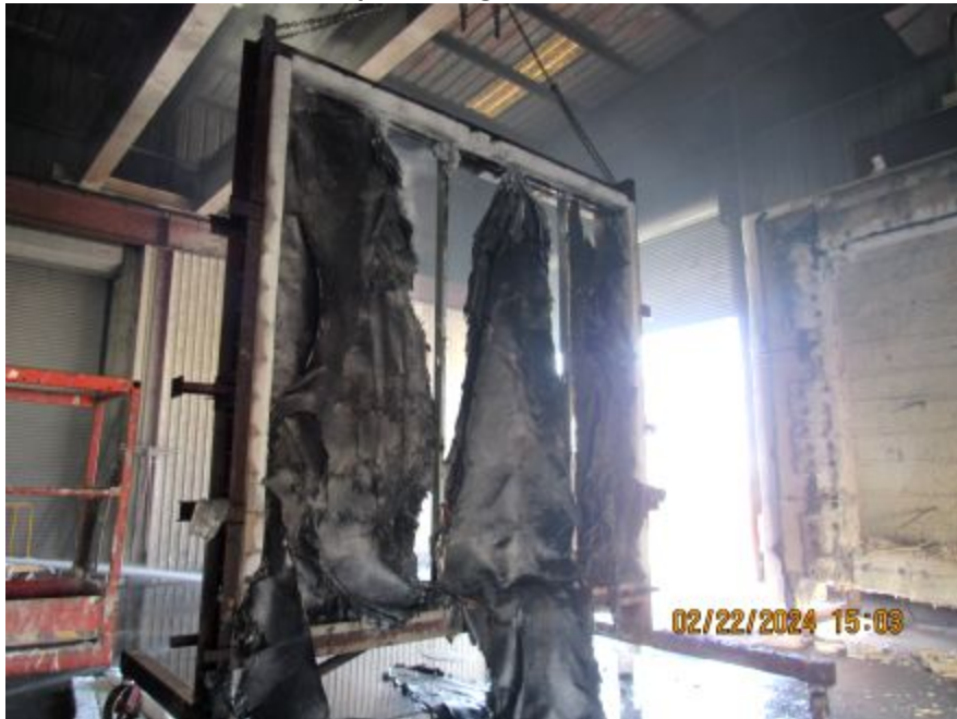
Photo No. 16 Sample Post Hose-Stream
