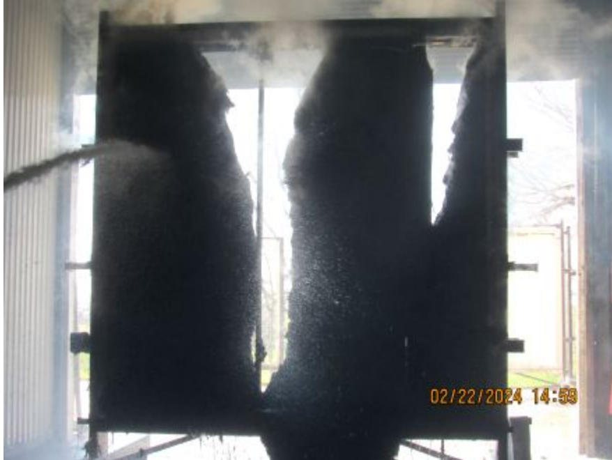
Photo No. 15 Sample During Hose Stream
