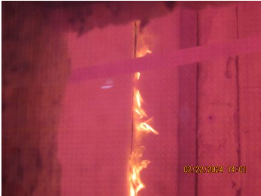
Photo No. 9 Flame in the Seam
