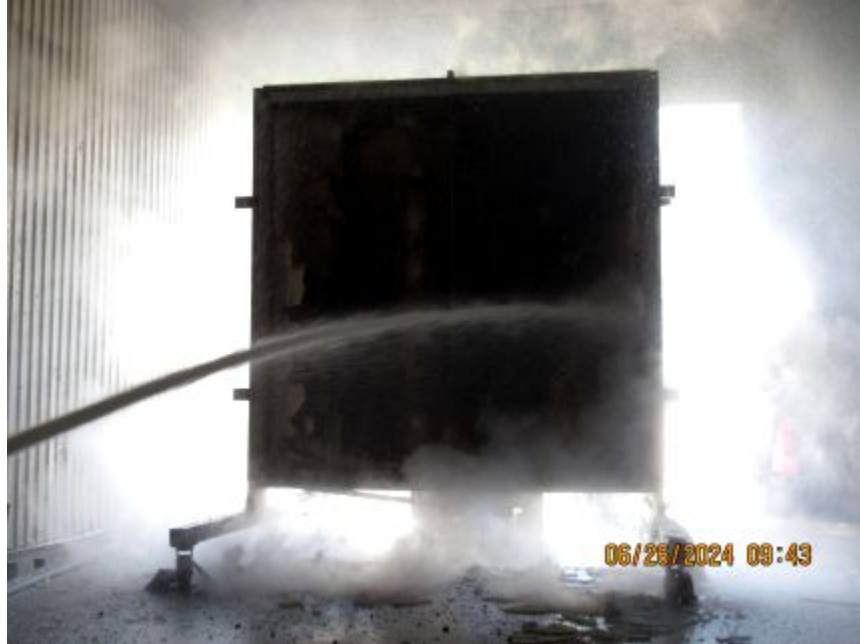
Photo No. 29 Hose Stream Re-Test
